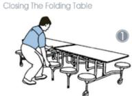
Release locking bar by pressing down on the table surface, with right hand lift clear the lock.
